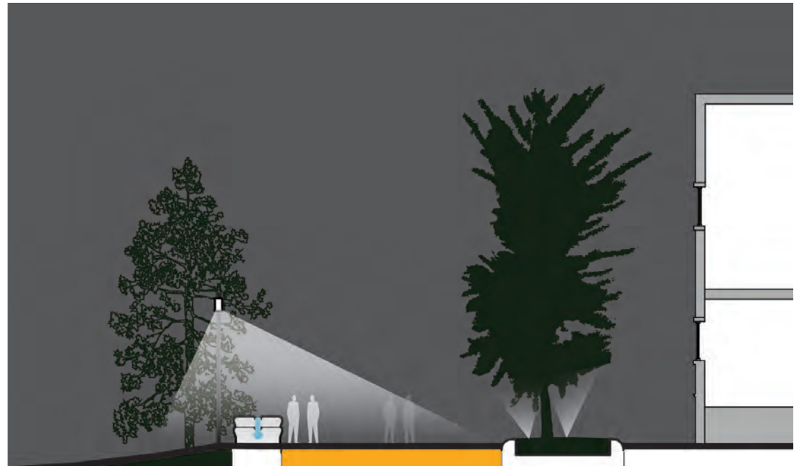
SECTION OF PATH LIGHTING AT LANCASTER WALK
